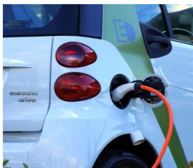
**Rapid chargers** are available as AC and DC. AC chargers are rated at 43kW and Rapid DC are usually 50kW. Both will achieve an 80% charge in around 30 minutes. Rapid DC chargers have two different connectors – CCS and CHAdeMO. Tesla Superchargers are also Rapid DC and currently charge at around 120kW!
